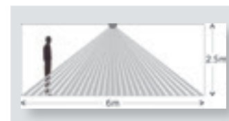
Cone shaped detection pattern. Optimum mounting height of 2.5m, gives detection diameter of 6m
